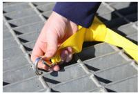
**4.** Pull the carabiner side through until the strap is tight and attach the carabiner to the grate. Repeat steps 3 and 4 for the other high visibility strap.
