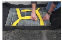
**3.** Take the carabiner from one of the high visibility straps and pull it through the loop of the other end of that same strap. Pull it tightly and attach the carabiner to the grate. Repeat for the other strap.
